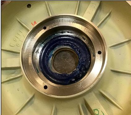
Figure A6: Lubricant retained in end bracket.
