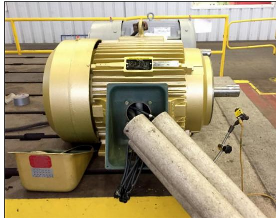
Figure A4: Incoming no-load test in service center.
