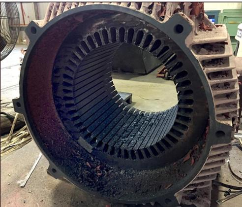
Figure A13: Stator with windings removed.
