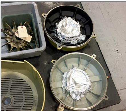
Figure A7: End brackets wrapped to protect retained grease.
