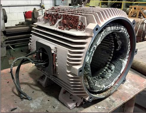
Figure A12: Stator winding post burnout process.
