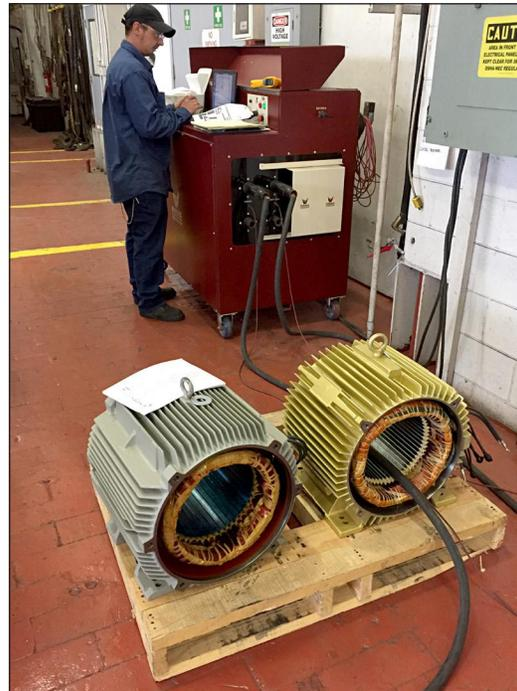
Figure A15: Stator core loss test.
