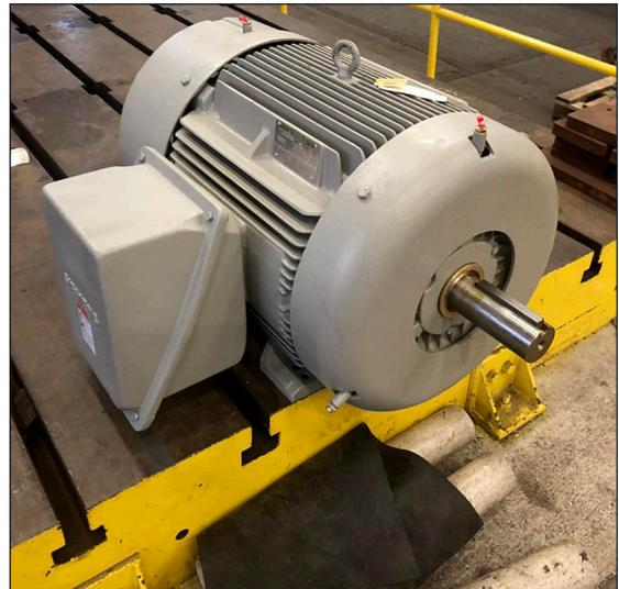
Figure A19: Motor after outgoing run test in service center.
