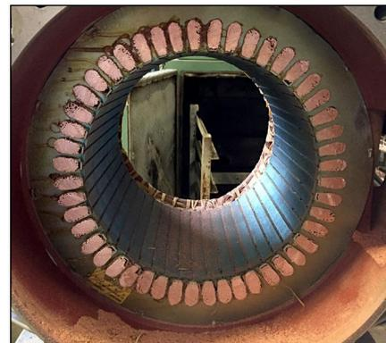
Figure A10: Stator winding extension cut off in preparation for burnout process.
