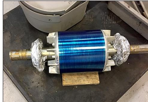
Figure A8: Rotor bearings wrapped to protect bearings and retained grease.
