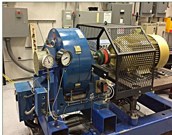
**Figure 1-1. Motor being dynamometer tested at Advanced Energy.**
