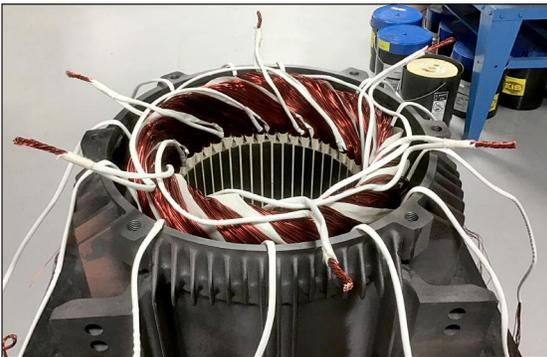
Figure A17: Stator connections being made.
